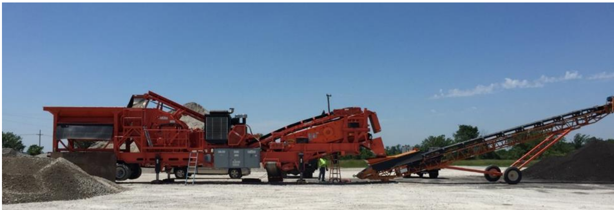
Figure 1. RAP Crushing/Screening Unit (courtesy HRG)
