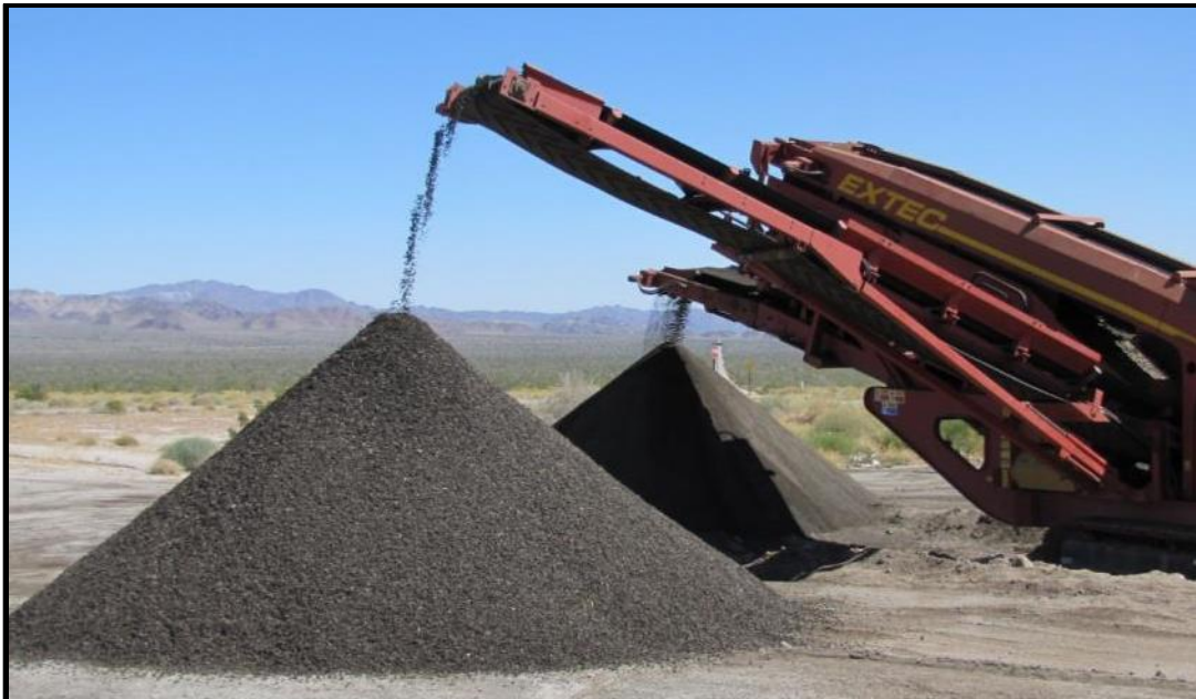
Figure 5 Fractionating RAP (Courtesy ARRA)
