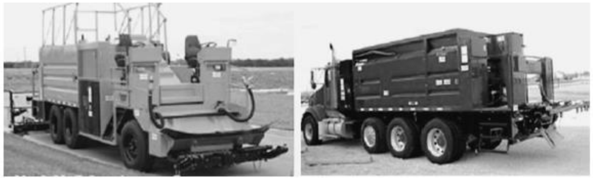
Figure 1 —Continuous Front-Loaded Self-Propelled (Left) and Truck-Mounted (Right) Micro Surfacing Mixing Machines ( Gransberg, 2010 )
